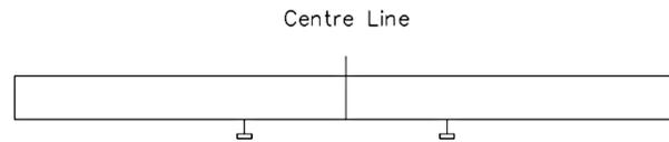
Fork positions must be centred on the panel with as wide a spread as possible when using forklifts/telehandlers.
