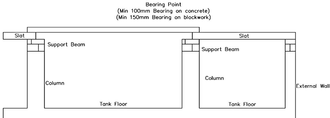
The section through a typical tank above shows the standard bearing detail, the units must bear at least 100mm on concrete or 150mm on blockwork. Care should be taken to ensure that loading capacities are never exceeded, either during construction or during lifespan.
