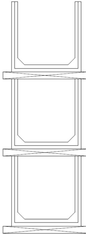
(Section view – stacking of Slurry Channels)
