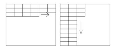
Laying direction can be achieved in either of the directions shown above, care must be taken to avoid falls from height. It is recommended to install edge protection on all open edges as construction progresses.
