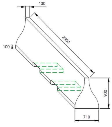
The barrier has **2nr 250mm deep x 100mm** wide forklift recesses to facilitate easy handling. Can be painted upon request.
