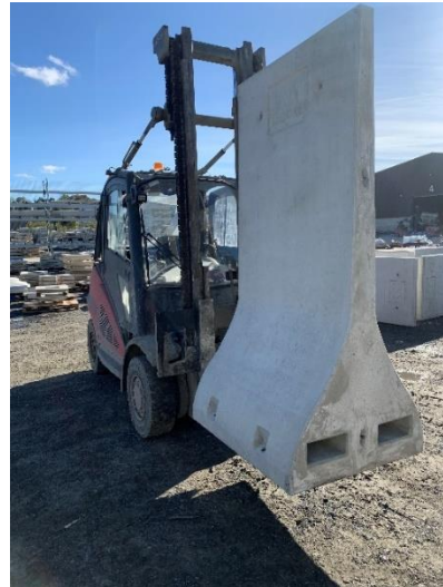
2.4m high Bunker Wall
