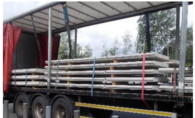
Timber spacers placed \frac{1}{5} of overall length from product ends.
