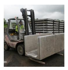
Lift channels using forklift toes
