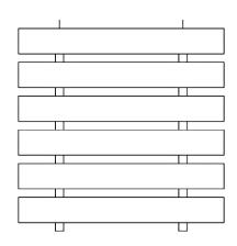
Fork positions must be centred on the panel with as wide a spread as possible when using forklifts/telehandlers.
