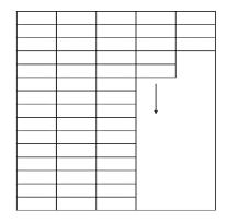
Laying direction can be achieved in either of the directions shown above, care must be taken to avoid falls from height. It is recommended to install edge protection on all open edges as construction progresses.
