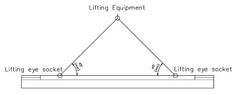
Slings must be sufficiently spread to balance the unit
