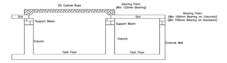
The section through a typical tank above shows the standard bearing detail, the units must bear at least 100mm on concrete or 150mm on blockwork. Care should be taken to ensure that loading capacities are never exceeded, either during construction or during lifespan.
