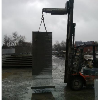
Raised with 2x lifting pins
