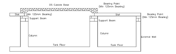
The section through a typical tank above shows the standard bearing detail, the units must bear at least 100mm on concrete or 150mm on blockwork. Care should be taken to ensure that loading capacities are never exceeded, either during construction or during lifespan.
